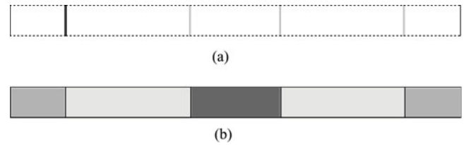
Fig. 1. Finite Element conditions. (a) Boundaries (bold line: incident wave, dotted: Neumann boundary condition, grey: continuity). (b) Subdomains (from left to right: PML / air / shielding sheet / air / PML).
