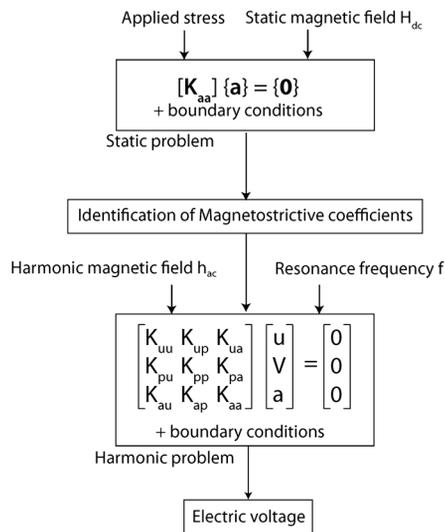
Fig. 3. Modeling procedure for the ME sensor, the mechanical boundary conditions are considered in both static and harmonic problems.
