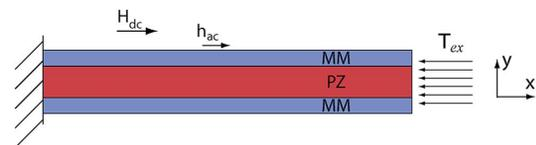
Fig. 1. ME sensor configuration: trilayer structure of magnetostrictive (MM) and piezoelectric (PZ) materials subjected to a uniform magnetic excitation  $\mathbf{h}_{ac}$  superimposed to a static magnetic field  $\mathbf{H}_{dc}$ . The mechanical boundary condition is a uniaxial stress  $\mathbf{T}_{ex}$  applied on the right side of the sensor, the left side being clamped.
