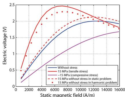
Fig. 4. Influence of the applied stress on the ME effect, according to different approximations.
