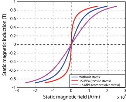
Fig. 2. Magnetic induction curves in the absence of stress and under uniaxial compressive and tensile stress (magnitude 15 MPa).
