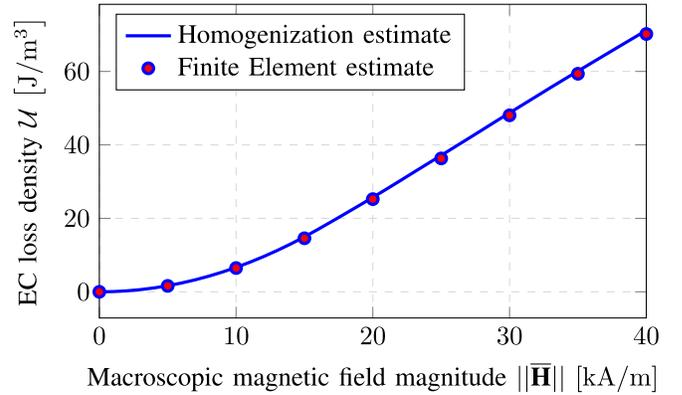
Fig. 6. EC losses density of a cubic cell of SMC as a function of macroscopic magnetic field magnitude  $\|\bar{\mathbf{H}}\|$ . Frequency: 1 kHz.
