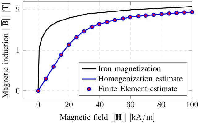
Fig. 4. Macroscopic magnetization of a cubic cell of SMC.
