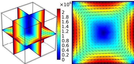
Fig. 5. FE result: EC distribution (unit:  $A/m^2$ ) in slices of the unit cell at  $t = 0.5$  ms (see Fig. 3, frequency: 1 kHz).
