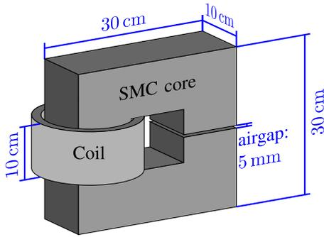
Fig. 7. Geometry of the magnetic circuit made of SMC with its coil (inner radius: 7.5 cm, outer radius: 9 cm) for the 3-D FE study.
