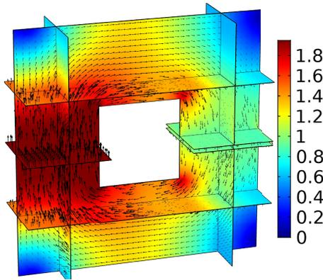
Fig. 8. Magnetic induction  $\mathbf{B}$  distribution (unit: T) in different slices of the magnetic core when the current in the coil is at peak value.
