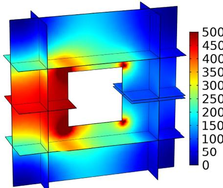
Fig. 9. EC loss density  $\mathcal{U}$  (unit:  $\text{J}/\text{m}^3$ ) in different slices of the magnetic core. Frequency: 1 kHz.
