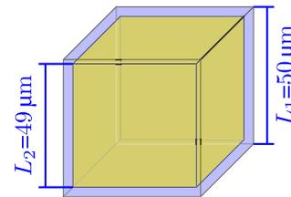
Fig. 1. 3-D unit cell of SMC: a cubic particle of ferromagnetic material (in yellow) is perfectly insulated electrically by a dielectric layer (in blue).
