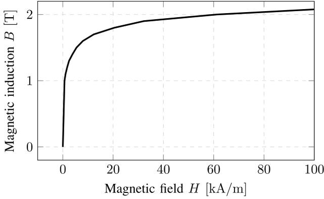
Fig. 2. Magnetization curve of iron [11].
