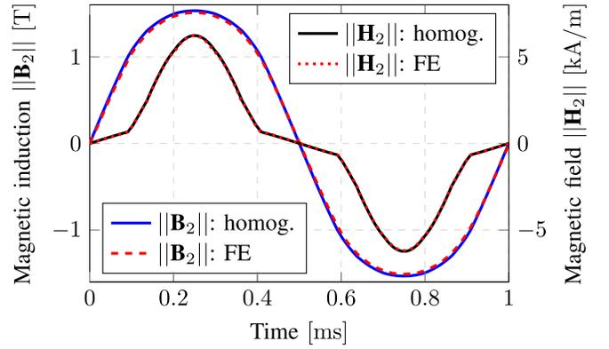
Fig. 3. Time evolution of magnetic field  $\|\mathbf{H}_2\|$  and magnetic induction  $\|\mathbf{B}_2\|$  evaluated at the center of the iron particle when a 1 kHz sinusoidal macroscopic magnetic field  $\bar{\mathbf{H}}$  (magnitude: 30 kA/m) is applied to the unit cell.
