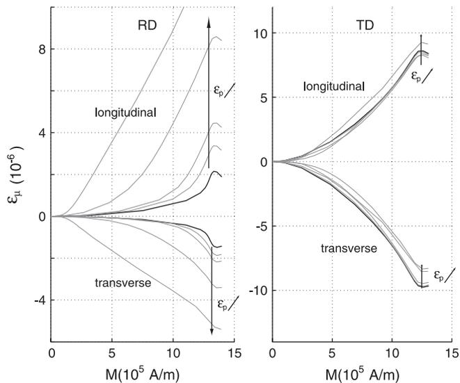
Fig. 4. Multiscale model: magnetostrictive behavior.
