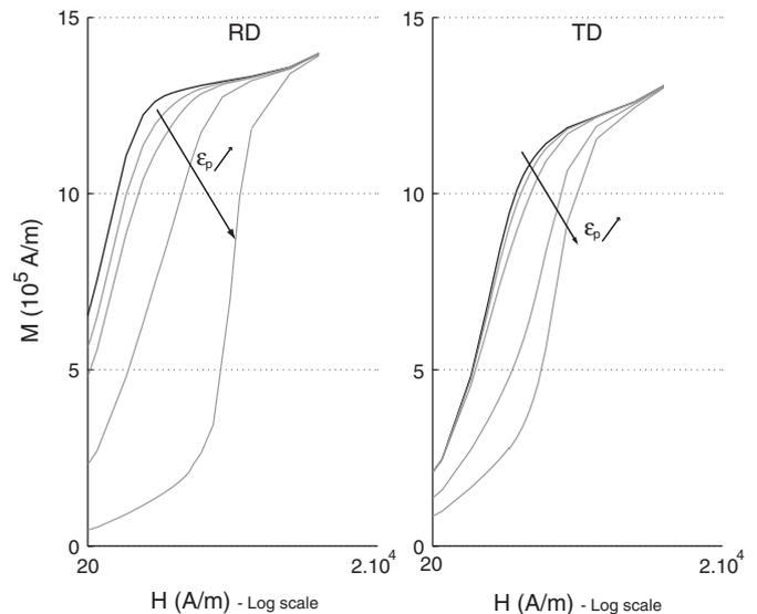
Fig. 3. Multiscale model: magnetization behavior.
