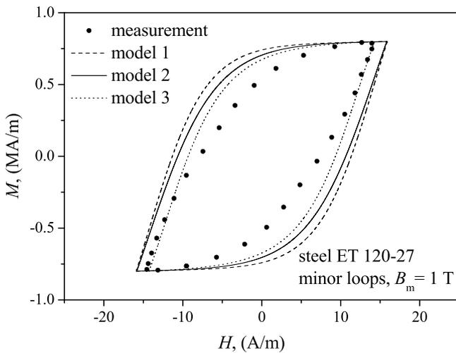
**Figure 5.** Minor hysteresis loops for the grain-oriented steel,  $B_m = 1.0$  T.
