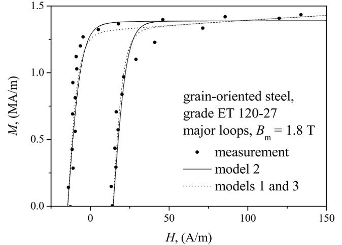
**Figure 3.** Major hysteresis loops for the grain-oriented steel.
