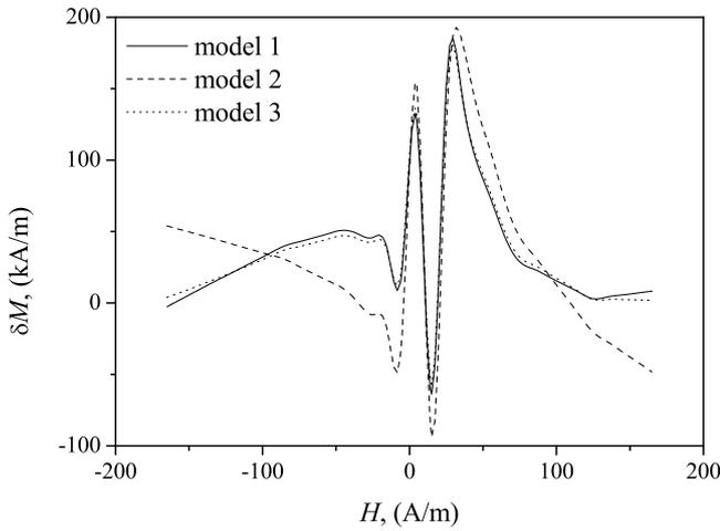
**Figure 4.** Deviations between the measured and the modelled data points belonging to the ascending branch of major hysteresis loop.
