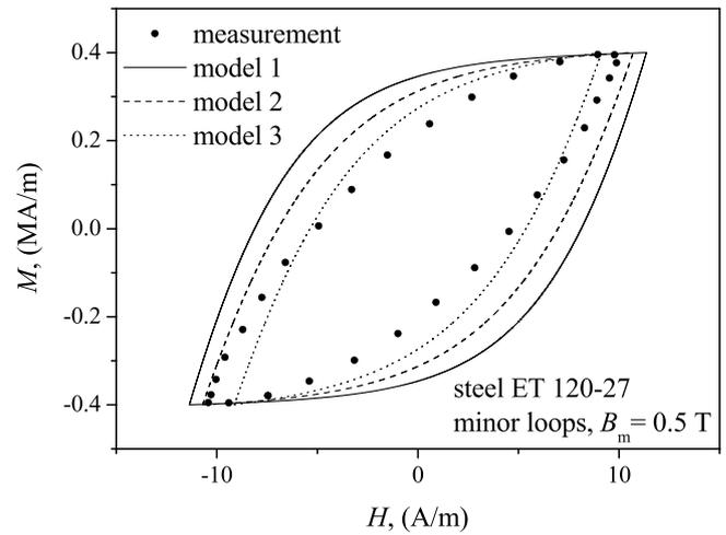
**Figure 6.** Minor hysteresis loops for the grain-oriented steel,  $B_m = 0.5$  T.
