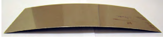
Fig. 6. Residual curvature of an iron-cobalt sheet after severe coiling curvature denotes internal stresses.
